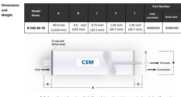
1. Each membrane elements upplied with one brine seal, one interconnector (coupler) and four o-rings. 2. All NE4040 elements fit nominal 4.0 inch (102 mm) I.D. pressure vessels.
